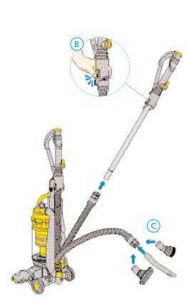
**B** To fit tools directly to hose, first extend the wand. Then press side buttons to remove wand handle from the hose.
